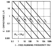
Figure 16. Free Running Frequency
